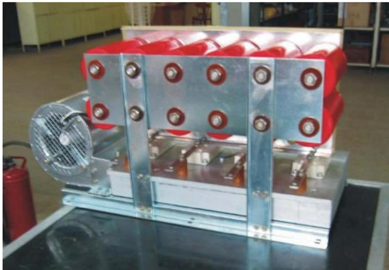
**Fig.9.** IGBT transistor bridge
